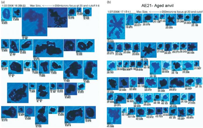
Figure 2. Images of ice crystals detected by Manchester University's Cloud Particle Imager mounted on the Airborne Research Australia's Egret Aircraft flying in anvils from Hector clouds over the Tiwi islands. (a) Crystals characteristic of those close into the main convective cell with large irregular crystals and aggregates including chain aggregates. (b) Crystals characteristic of an aged anvil featuring bullet rosette type crystals and small irregular crystals.
