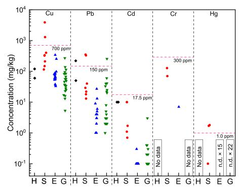
Fig. 3. Contaminant trace metal concentrations in four different biomass ashes (n.d.  $\times$  n – not detected in n samples; pink dotted line – Finnish limits for ash to be used as a forest fertiliser [5]; H – hardwood ash; S – softwood ash; E – eudicot straw ash; G – grasses straw ash). (For interpretation of the references to colour in this figure legend, the reader is referred to the web version of this article.)
