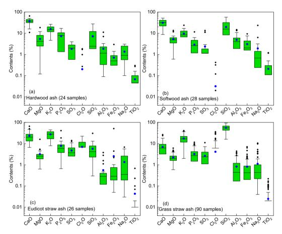
Fig. 2. Chemical composition of ashes derived from different types of biomass (shaded boxes show the median values and interquartile range; tails indicate  $1.5 \times IQR$ ; • mean value; • outliers).
