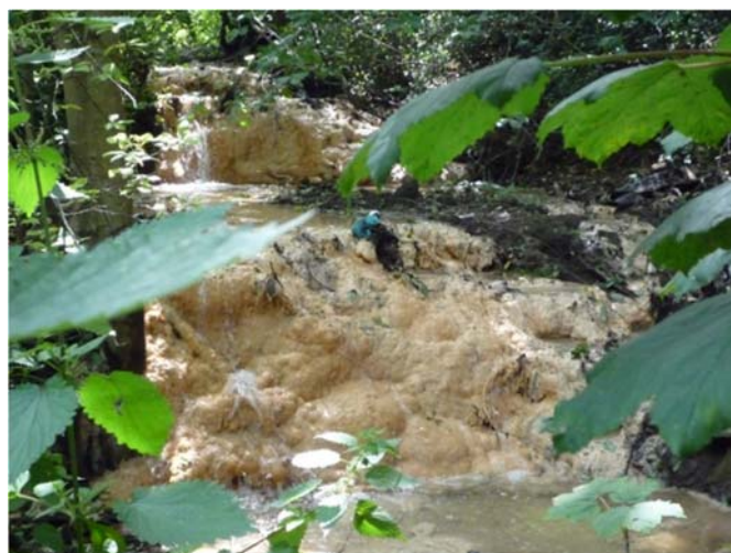
Figure 3: Calcium carbonate deposits downstream of the former Consett Steelworks – the end product of slag leaching and atmospheric CO 2 uptake (water pH >11.0).
