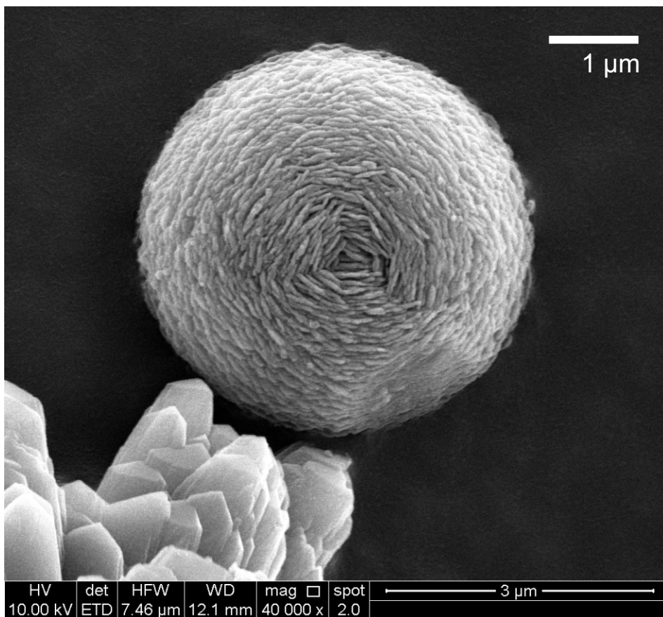
Figure B.10: Vaterite ball observed after 6 h in the 40 °C experiment
