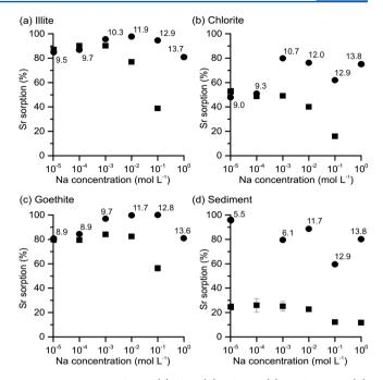
**Figure 1.** Sorption of Sr to (a) illite, (b) chlorite, (c) goethite, and (d) sediment as a function of Na concentration in a background of NaCl (squares) and NaOH (circles). The pH of the NaOH systems is annotated to clearly show the increase in pH with increasing concentration. All data points represent the average of a triplicate sample. Error bars are not shown where they were smaller than the symbol used.
