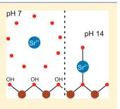
that at highly alkaline pH (>12.5) Sr was forming inner-sphere complexes on the surfaces of all minerals. This specific adsorption of the Sr (as  $SrOH^+$ ) explains why it was still adsorbed to the minerals under very high ionic strength conditions and was not outcompeted by Na.
