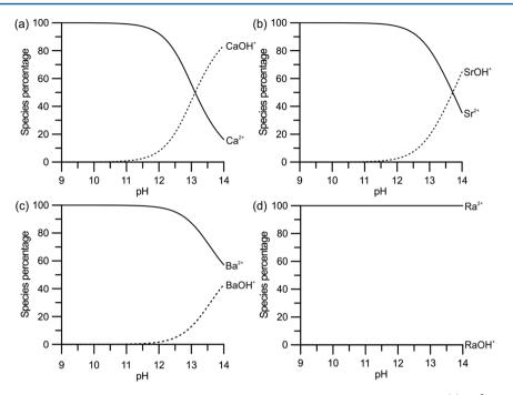
Figure 6. Speciation of four alkali earth elements as a function of pH determined by PHREEQC modeling: (a)  $Ca^{2+}$  and  $CaOH^+$ ; (b)  $Sr^{2+}$  and  $SrOH^+$ ; (c)  $Ba^{2+}$  and  $BaOH^+$ ; and  $CaOH^+$ ; (b)  $Sr^{2+}$  and  $SrOH^+$ ; (c)  $Ba^{2+}$  and  $BaOH^+$ ; and  $CaOH^+$ ; (b)  $Sr^{2+}$  and  $SrOH^+$ ; (c)  $Ba^{2+}$  and  $BaOH^+$ ; and  $CaOH^+$ ; (b)  $Sr^{2+}$  and  $SrOH^+$ ; (c)  $Ba^{2+}$  and  $BaOH^+$ ; (c)  $Ba^{2+}$  and  $Ba^{2$
