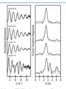
**Figure 2.** Sr k-space EXAFS and accompanying Fourier transform of Sr sorbed to ilite at (a) pH 8.9, (b) pH 9.2, (c) pH 13, and (d) pH 14. Solid lines are background subtracted data, and dashed lines are refined model fits.
