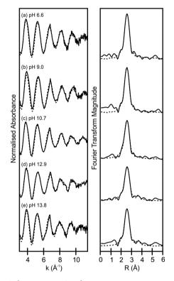
Figure 3. Sr k-space EXAFS and accompanying Fourier transform of Sr sorbed to chlorite at (a) pH 6.6, (b) pH 9.0, (c) pH 10.7, (d) pH 12.9, and (e) pH 13.8. Solid lines are background subtracted data, and dashed lines are refined model fits.
