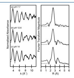
Figure 4. Sr k-space EXAFS and accompanying Fourier transform of Sr sorbed to goethite at (a) pH 7.7, (b) pH 12.6, and (c) pH 14.0. Solid lines are background subtracted data, and dashed lines are refined model fits.
